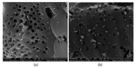
Figure 2. SEM pictures of activated carbon fom coal (a) and (b) palm shells (10,000-fold magnification)
