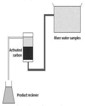
$\textbf{Figure. 1} \ \textbf{Schematic diagram of Experimental set up} \\$
